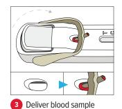
Rotate the **blood collection tube** over the **blood transfer zone** allowing it to lock into position.
